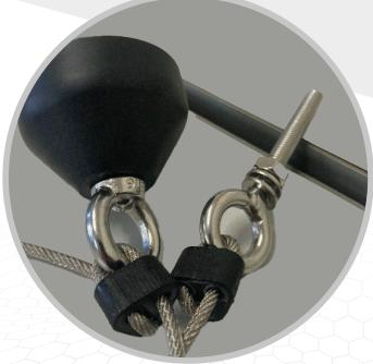
2. Adjustment of the wire rope length. 4m of flexible PVC coated SS wire lanyard is provided with each rip switch, whish is adjusted to provide flexibility for belt width, point of attachment and tensioning. 3 tensioners are provided, and the wire rope can be adjusted by pushing the wire rope through these thimbles until the desired length is reached.
